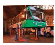
interconnecting cables helping to reduce health and safety issues associated with slips, trips and falls. Ancillary devices will also be on display, including tall support stands and a transmission jack, while Alexander Dennis will be helping to demonstrate the flexibility and effectiveness of the Somerstotalkare cable-free lift range by providing an Enviro 400 double-decker bus.
